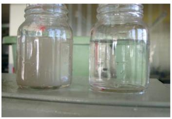
Water sample before and after chamber filtration
