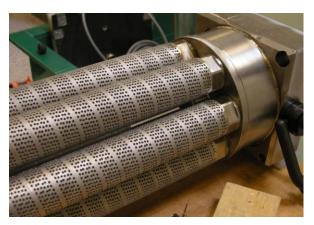
AMFM internals showing high-capacity, sintered metal filtration media (0.5 micron rating)
