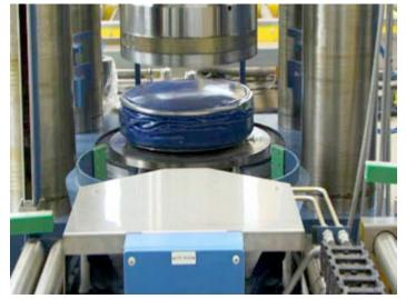
Crumble drum after compaction
