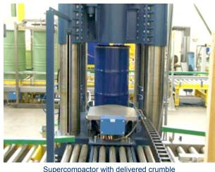
Supercompactor with delivered crumble drum of radioactive waste
